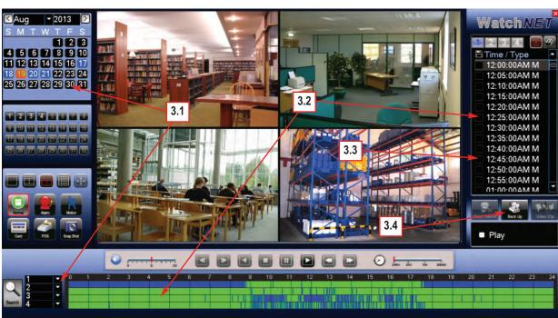
Insert USB Drive to the NVR before starting back up process
