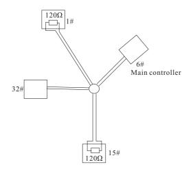
In such circumstances the factory recommends the usage of RS485 distributor. The distributor can change the star configuration connection to the mode of connection stipulated in the RS485 standards. The new connection achieves reliable data transmission. (Refer to Picture 10-4.5).
