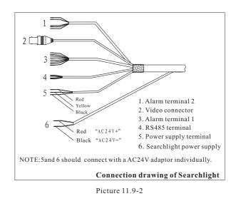
Please connect cables refer to the attached tag. Detail connection refer to below list.
